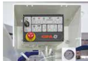
REAR CONTROL PANEL Control panel positioned on the rear side (only for closed loop circuit pumping unit).
