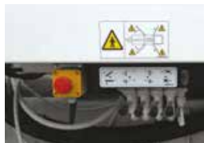
HYDRAULIC OUTRIGGERS CONTROL Hydraulic controls on both sides of truck pump. The machine emergency stop is also positioned nearby.
